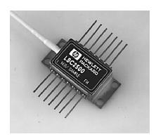
heatsink mounting flange is incorporated into the industry standard 14 PIN package.
